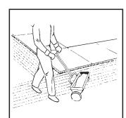
Close the spreader when you stop walking or make turns to avoid uneven coverage. gaps in coverage.
